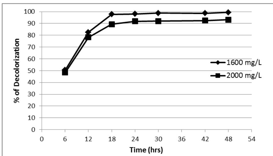
Figure 6. Effect of contact time on decolorization of BR 46 dye by *Enterobacter cloacae* sp. A3.
